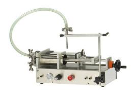
Tabletop Piston Liquid Filling Machine FP-100 is the best candidate with the consideration of budget. The volumetric piston filler draws liquids and other low viscosity products such as oils or juices directly from a tank or drum It is the simple design, low failure rate and fully operated by air.
